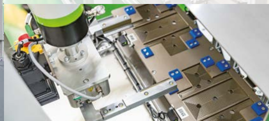
6-axis robot arm and palette with RFID (radio frequency identification)
